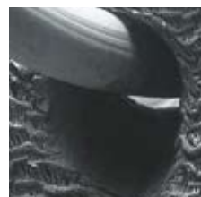
SEM showing monofilament suture through the needle hole made in a GORE-TEX® Vascular Graft by a TT-12 equivalent needle.
