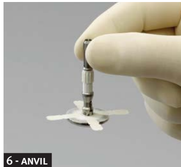
6 - ANVIL Slide the centering hole over the post of the anvil with the adhesive backing paper facing the anvil.
