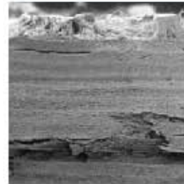
Scanning electron microscopy (SEM) comparison of the cross-sectional ePTFE structure of GORE DUALMESH® Biomaterial to BARD® DULEX mesh (50x magnification).
