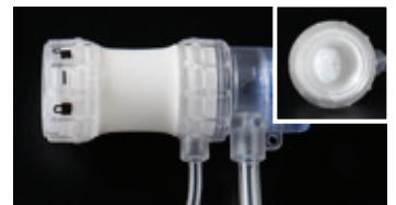
Figure 2. Valve after pressurization
